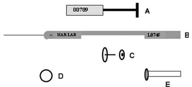
Fig. 2. Tags for marking individual squid, *Loligo forbesi* in captivity. (A) Anchor tag (25 mm); (B) soft plastic band tag (95 mm long and 3 mm high); (C) pin tag (5 mm); (D) glued circles of white sheet plastic (5 mm); (E) metallic rod (7.5 mm) used for burning marks.
