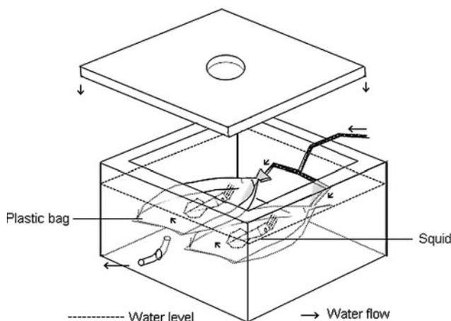
Fig. 1. Transport boxes design for holding individual *Loligo forbesi* after being caught by jigging.
