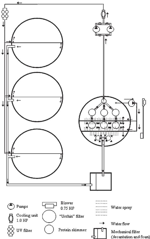
Fig. 3. Closed seawater system used for maintenance of *Loligo forbesi* during three culture trials.
